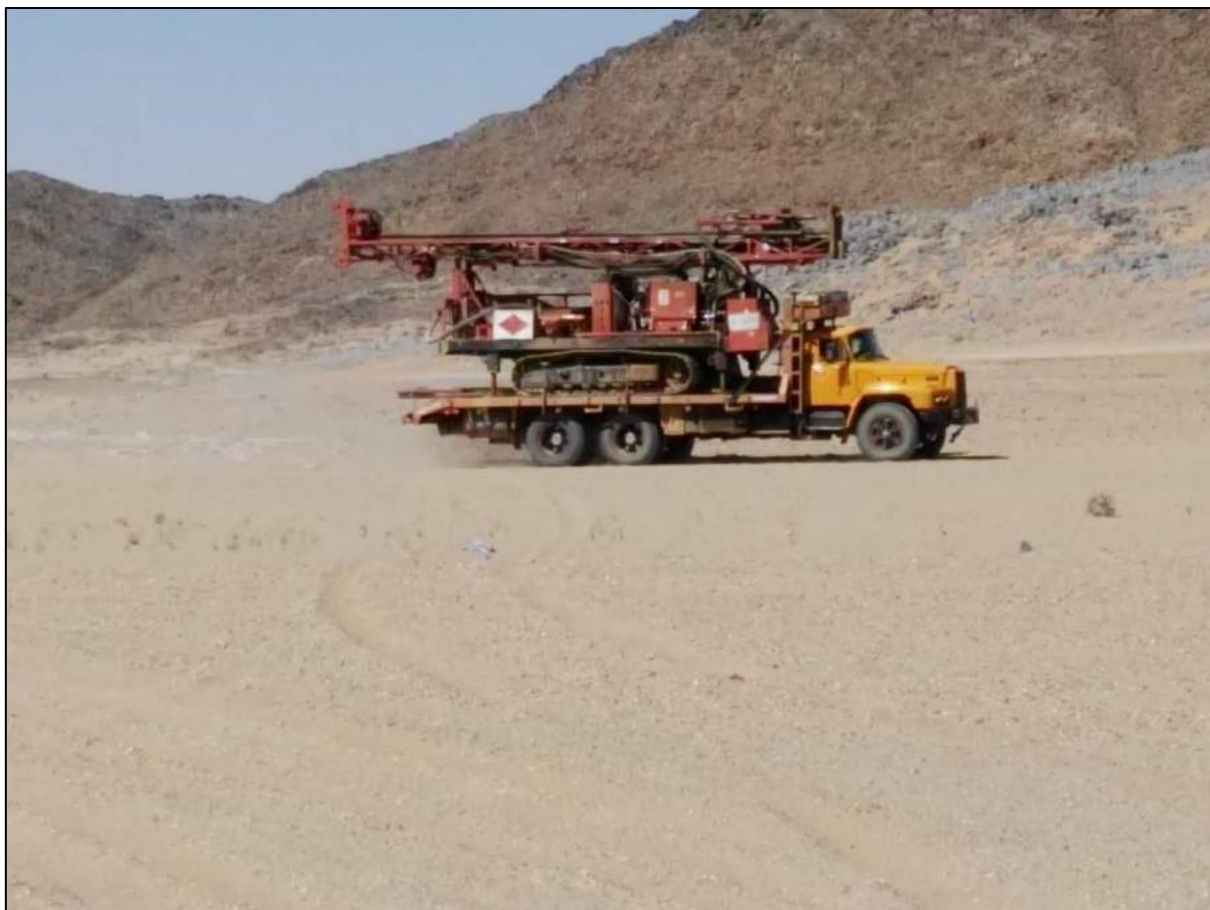
Figure 5.1 Transporting 20 t Reverse Circulation Drill Rig
